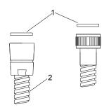
Put the washer(1) into each connector of hose(2). Connect handspray and wall-mount supply elbow or shower outlet with hose.
